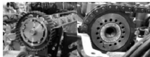
Fig. 2. Variable timing camshaft mounted on test engine.
